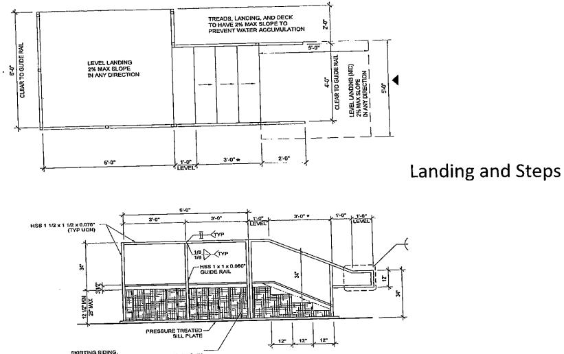
SKIRTING SIDING. BLOCK ALL EDGES. ATTACH WITH BI AT 6" OC EN AND 12" OC FN. AT EDGE CONNECTION TO TUBE STEEL USE #14 X 2" TEK SCREWS AT 6" OC
