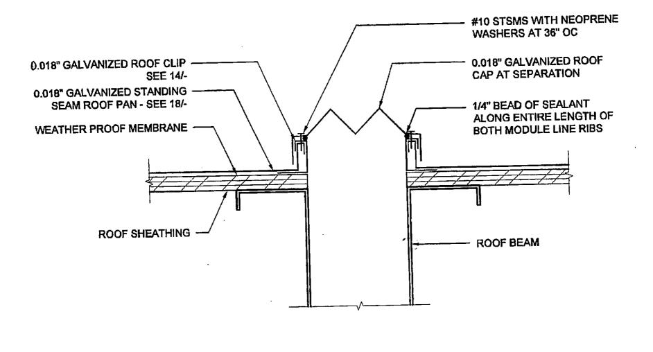
6" separation expansion cover at roof
